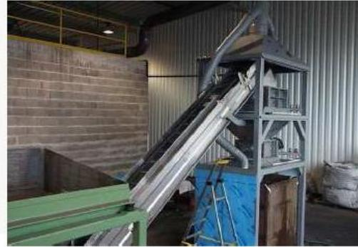
The organic lithium shredding process is specific because it needs a water flow in order to catch the solvent present in lithium batteries.
